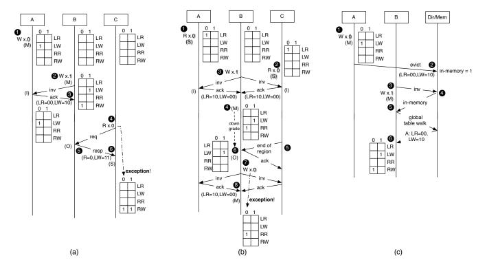
Figure 3: Examples: (a) In-cache operation; (b) In-cache operation with downgrade; and (c) Out-of-cache operation. Caches A, B and C access the same cache line x, which consists of two bytes. Letters in parenthesis show the MOESI coherence state.
